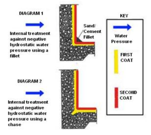
It is important not to mix more material than can be applied within 30 minutes at 20℃. recommended mixing ratio is approximately 2.5 to 3 parts Aqua-Stop to one part clean water by volume. It is recommended that the powder is added slowly to the water and mixed to a smooth lump free consistency.
